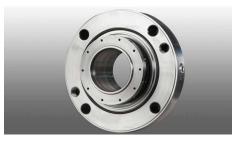
Mechanical seals type **LL9UC** are installed to seal shafts of sea water injection pumps installed at various FPSOs. p = 35 bar; t = +20 °C ... +60 °C (+68 °F ... 140 °F); n = 5,500 ... 6,000 min<sup>-1</sup>.
