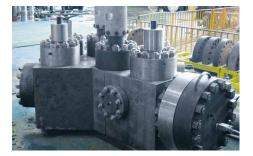
A manufacturer of drilling equipment uses EagleBurgmann RX **ring type joints**, specially designed to withstand high pressures, in its wellheads. Media: drilling sludge, water/sand mixture, dihydrogen sulfide, natural gas, heavy hydrogen sulfide. The RTJ also provide reliable sealing in extreme conditions. Operating conditions: p ... 1,370 bar (19,870 PSI); t ... 60 °C (140 °F).
