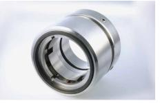
The pump stations along the 700 km pipeline which extends from the Sudanese oil fields of Baleela to Karthoum have 300 EagleBurgmann seals of type **HJ4**, in different versions, installed in Bornemann screw pumps. Suction pressure  $p = 4 \dots 50$  bar (58 ... 725 PSI);  $t = 29 \dots 70$  °C (84 °F ... 158 °F);  $n = 440 \dots 1,240 \text{ min}^{-1}$ ; viscosity of media: 990 ... 1,700 mm<sup>2</sup>/s.
