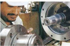
At Saudi Aramco in Saudi Arabia, an **SHV-D2/145-E1** from EagleBurgmann is used as a dual seal in a helico-axial multiphase pump from Sulzer. Operating conditions: Gas content ... 99 %; p = 60 bar (870 PSI); t = 80 °C (176 °F); n = 4,000 min<sup>-1</sup>.
