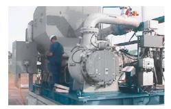
In Venezuela's Zuata field, a Bornemann twin screw multiphase pump has been operating with EagleBurgmann's **HSHJ97GS1/100-E1** (API Plan 32) single seal since 1998. Operating conditions: Gas content ... 98 %; p ... 25 bar (363 PSI); t = 93 °C (199 °F); n = 1,660 min<sup>-1</sup>.
