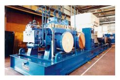
The ESPO (East Siberia – Pacific Ocean) pipeline operated by Transneft in Russia features EagleBurgmann **SHPVI1-D** dual seals in Sulzer's pipeline pumps. The barrier fluid is not oil, but water. Sixty dual highpressure seals for the main pipeline pumps and 24 API Plan 53B barrier systems with air-blast heat exchangers have been provided for the ESPO project. Operating conditions:  $p = 10 \dots 78$  bar (145 ... 1,131 PSI); t ... 50 °C (122 °F);  $n = 1,540 \dots 2,845 min^{-1}$ .
