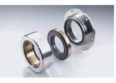
In Korea, Latin America and Middle East, our dual seals of type **LB800/EKU750** are applied on screw compressors. Operating condition:  $p = -0.01 \dots 5.7$  bar (-0.2 ... 82.6 PSI); t = 34.9 °C ... 205 °C (94.8 °F ... 401 °F);  $n = 1,859 \dots 11,281 \text{ min}^{-1}$ . Medium: Gasified LNG with high percentage of methane.
