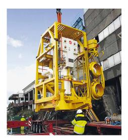
Subsea multiphase pumps sealed with EagleBurgmann **SH18/115** mechanical seals. Operating conditions: Media: oil-water-gas mixture; gas content:  $25 \dots 70 \%$ ; suction pressure:  $p = 5 \dots 70$  bar ( $73 \dots 1,015$  PSI); rotational speed: n = 4,200 min<sup>-1</sup>.
